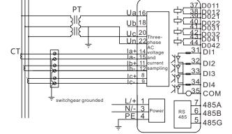
Angle system: no voltage transformer (PT), 3 current transformers (CT) (Device is set to 2LL3Ct)
