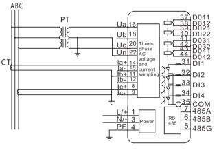
Angle system: use 2 voltage transformers (PT), 2 current transformers (CT) (Device is set to 2LL2Ct)
