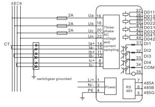
Quad-line star system: direct wiring without voltage transformer (PT) (device set
