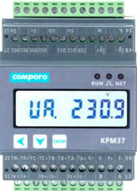
KPM37 Three Phase Rail Smart Power Meter adopts DIN 35MM rail type installation structure and LCD display. It integrates three-phase electric parameter measurement, 2-31st harmonic analysis and time statistics. KPM37 default communication is Modbus-RTU by RS485 interface. WiFi, 4G, Lora communication are optional. The meter can also expand 2-way digital input and 2-way relay output, 4-way temperature measurement and 1 way residual current measurement.
