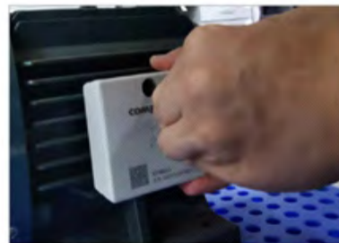
Figure 7. Intelligent temperature vibration sensor flat bottom fixing diagram
